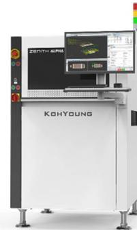
6. **KY8030-3:** *Industry's Fastest True 3D Solder Paste Inspection Solution*
