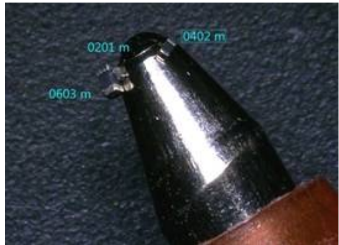
Figure 1: Using a ballpoint pen for reference, the image compares 0201 metric (008004 imperial) component with an 0402 metric (01005 imperial) and an 0603 metric (0201 imperial) component [image courtesy of ASM Assembly Systems GmbH]
