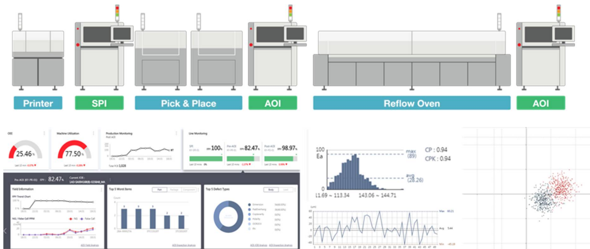
Image 1: Example of a line configuration to improve yield with multipoint data correlation
